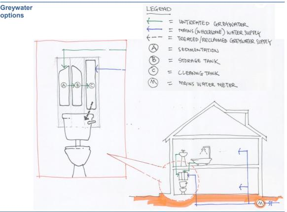
Figure 3. Example short retention systems schematic
