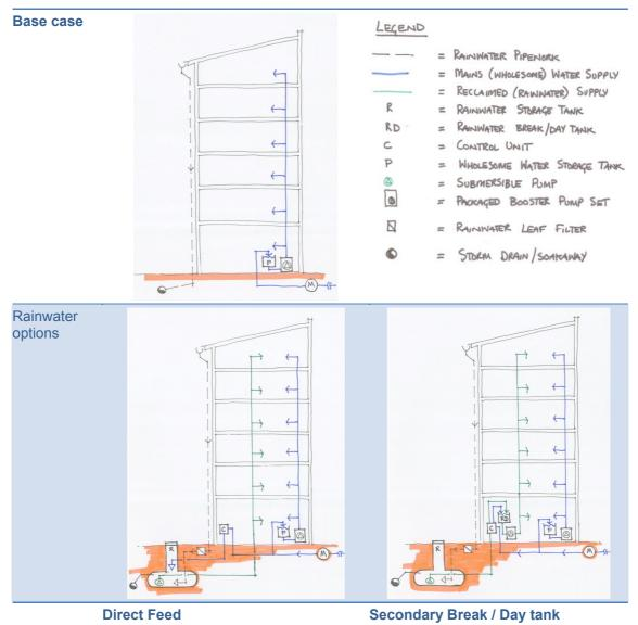
Figure 2. Options for pumped supply in larger buildings
