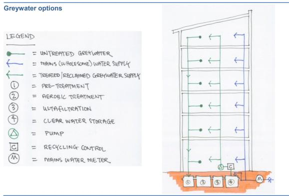
Figure 5. Example bio-mechanical systems schematic
