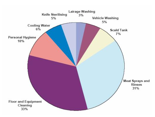
Figure 1 Typical water balance for areas in a pig abattoir
